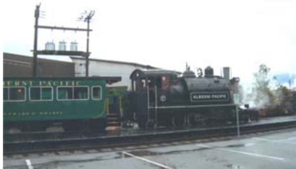
1929 Baldwin 2-8-2T steam engine
